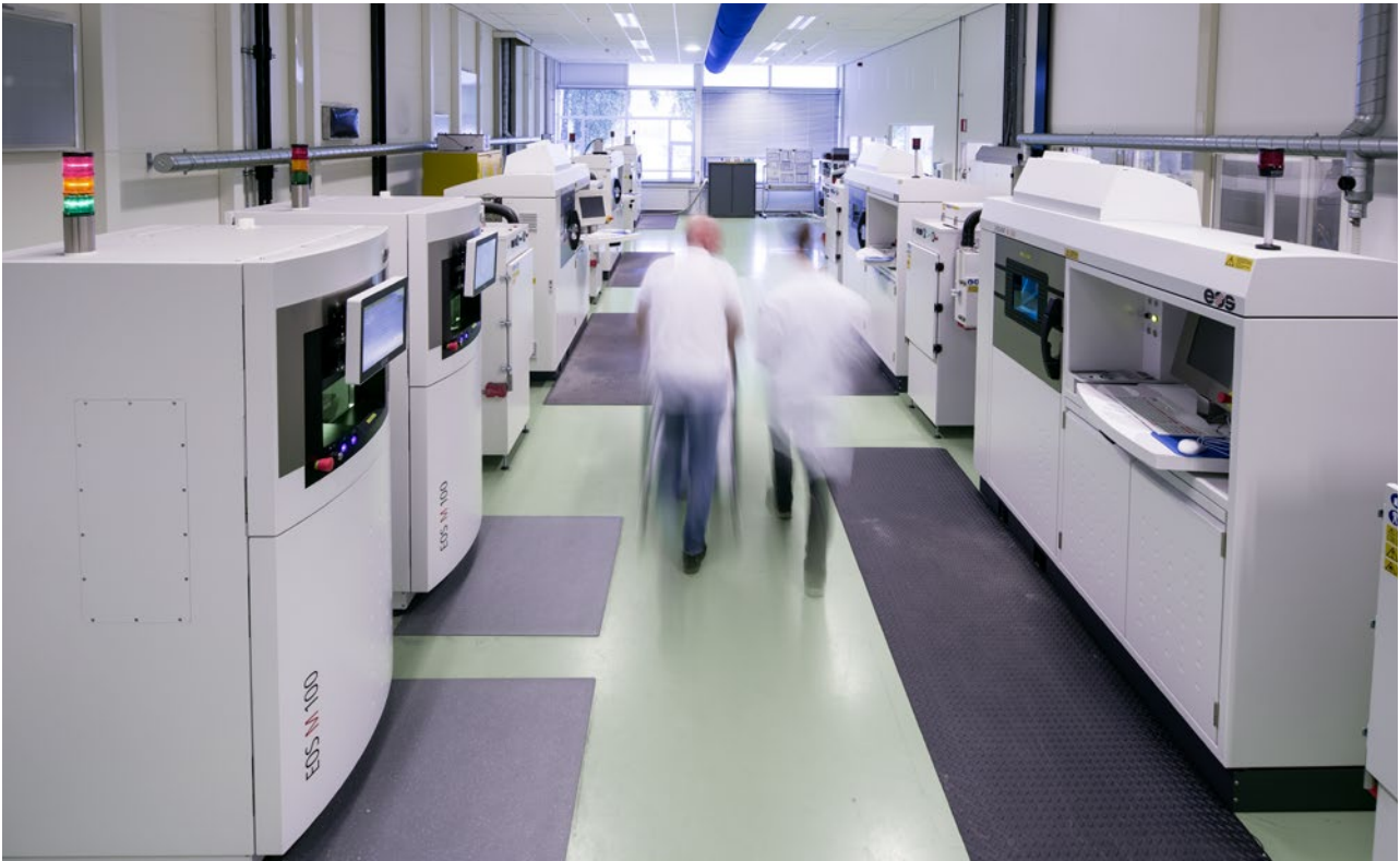
DMLS factory for mass production of high-precision 3D-printed tungsten parts.
