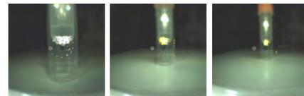
The **final augmented images**, thresholded and smoothed, show that the activity blob is scaled down with increasing distance.
