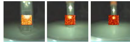
For each of the distances, the gamma activity image patch of the central pinhole is **overlaid on top of the optical image** of its camera.
