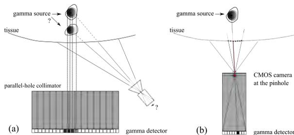
In order to overlay the two modalities, the pinhole and the camera need the same opto-geometric mapping and aligned viewing axes to produce a corresponding **perspective projection** (b). This cannot be achieved using an orthographic projection without knowing the depth of the source (a).
