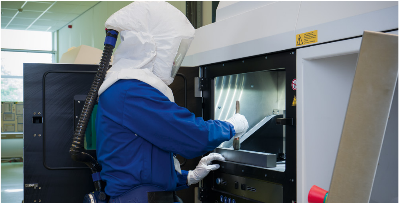
Removing and cleaning 3D-printed tungsten parts
